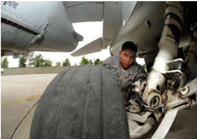
Airman 1st Class John Kulwatno, Aircraft Maintenance Unit crew chief, performs a basic post-and pre-flight inspection on an F-16 Fighting Falcon July 7 at Aviano Air Base, Italy.
