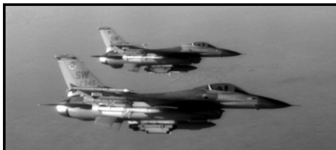
77th & 78th FS F-16s on patrol Apr. 7, 1998 near the Iraqi border as part of Operation Southern Watch. They are carrying Low Altitude Navigation and Targeting Infrared for Night (LATNTIRN) systems and are fitted with AIM-9 Sidewinder, AGM-88 Harm (mid-wing) and AIM-120 AMRAAM Slammer missiles on the wing tips. USAF Photo
