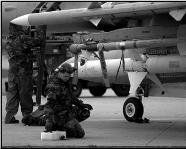
SSgt Rob Anson replaces the argon bottle in an AIM-9 missile on Apr. 19, 1999. Anson is deployed with the 78th EFS to Aviano AB, Italy in support of Operation Allied Force.
